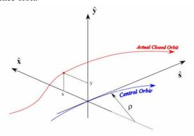
Figure 2: Coordinate system used to describe the motion of the beam in an accelerator.
