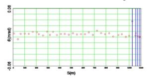
Figure 4: Kick strengths calculated from the orbit difference between MI at 150 GeV with LAM52 and V701 ramping and MI at 8 GeV before the LAM52 and V701 magnet bus work. The blue lines indicate the location of simulated kicks.
