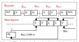
Figure 1: The lattice in Recycler ring around one of the Main injector Lambertson (L) and C-magnet (C). RGF and RGD represent the gradient magnets, F and D represent focusing and defocusing quadrupoles. PS is Power Supply.  $K_{s51}$ ,  $K_{s52}$ ,  $K_{s53}$  and  $K_{s54}$  (in red) are simulated virtual kicks.
