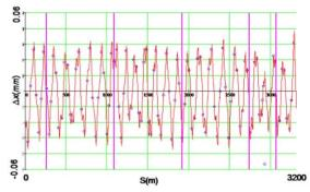
Figure 3: Orbit difference between MI at 150 GeV with LAM52 and V701 ramping and MI at 8 GeV before the LAM52 and V701 magnet bus work. Blue circles are measured values, red line is the fitted value. BPMs from RR-302 to RR-308 are masked. Noted here most measured values of those BPMs are out of range.
