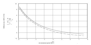
Figure 1: The calculated longitudinal IBS diffusion rate as a function of the rms beam momentum spread in the Recycler for a coasting beam of  $100\times10^{12}$  antiprotons with a constant 5  $\pi$  mm-mrad emittance. The solid line is modeled from Ref. [2]; the dashed line is the round-beam, zero-dispersion, smooth approximation.
