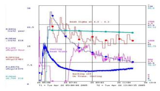
Figure 7: Demonstration of IBS-assisted longitudinal cooling: the rms momentum spread was kept at about 4 MeV/c as the beam cooled longitudinally, so as to take advantage of small IBS rate.
