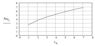
Figure 2: The value of the rms momentum spread in MeV/c, for which the longitudinal IBS heating vanishes, as a function of beam emittance (n, 95%) in  $\pi$  mm-mrad.
