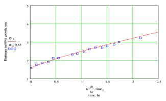
Figure 5: The transverse emittance evolution for a bunched antiproton beam  $(25 \times 10^{10})$ .
