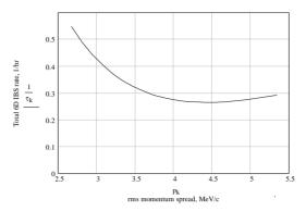
Figure 8: The total 6-D IBS heating rate for a  $100 \times 10^{10}$  coasting antiproton beam with a 4  $\pi$  mm-mrad emittance.
