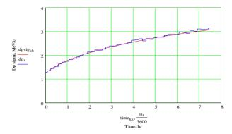
Figure 4: A comparison of the measured rms momentum spread (MeV/c) and the IBS model as a function of time for a coasting beam of  $100 \times 10^{10}$  protons.
