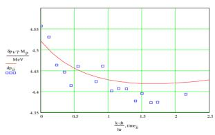
Figure 6: The longitudinal rms momentum spread (MeV/c) as a function of time (hours). The IBS model (solid line) has only one adjustable parameter – the vacuum-related transverse emittance growth rate.
