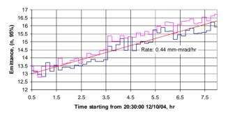
Figure 3: The transverse emittance (horizontal and vertical) evolution for a coasting beam of  $100 \times 10^{10}$  protons in the Recycler. The linear fit yields a growth rate of  $0.44 \, \pi$  mm-mrad/hr.
