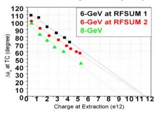
Figure 1(b)  $\Delta \varphi_s$  vs. the extracted beam intensity at RFSUM 1 and RFSUM 2 for the 6-GeV acceleration, and RFSUM for the 8-GeV acceleration are shown as the black, red, and green points respectively; and their linear-fit results are shown as the black, red, and green lines.
