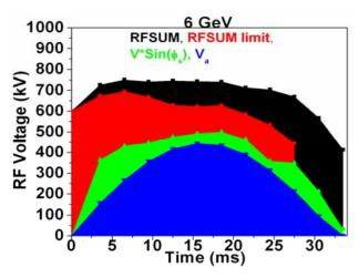
Figure 3(a) RFSUM, the lower limit for RFSUM, the effective accelerating voltage, and the accelerating voltage required by the magnet ramp are shown as the black, red, green, and blue curves respectively. All data were taken under similar conditions at the extracted beam intensity of  $5.1 \times 10^{12}$  protons when Booster was operated at the 6-GeV acceleration.
