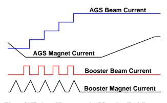
Figure 3: Timing of Booster and AGS cycles. Each Booster cycle is 200 ms long.
