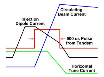
Figure 2: Typical timing at Booster injection.
