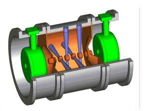
Figure 1: Cut-away view of the RT section of the linac comprising 5-gap CH cavity and two SC solenoids.
