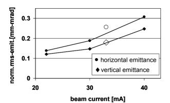
Figure 1: LEBT output emittance measurement results.
