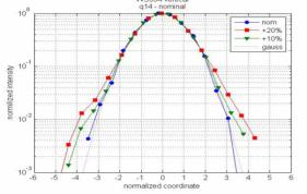
Figure 4: Effect of the MEBT matching quad change on the beam profile measured in the DTL. Blue circles – nominal "best match"; green triangles – nominal +10%; red squares – nominal +20%; dash – Gaussian fit.
