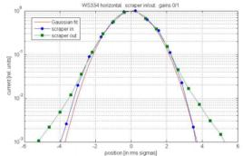
Figure 3: Effect of the MEBT scraper on the beam profile measured in the DTL. Blue circles – scraper is in; green squares – scraper is out; solid red line – Gaussian fit.
