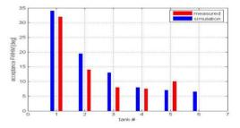
Figure 7: The measured (red) and simulated (blue) widths of the DTL acceptance curves vs. the tank number.
