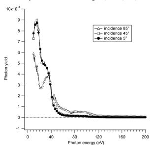
Figure 6: Photoelectron yield of the Al sample measured at incidence angles 85°, 45°, and 5°.
