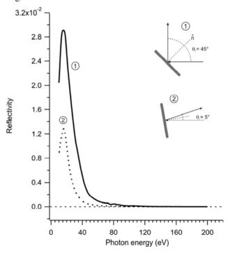
Figure 4: Reflectivity measurement with an incidence angle of 45° (1) and 5° (2).
