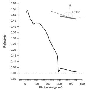
Figure 3: Reflectivity measurement with an incidence angle of 85°.
