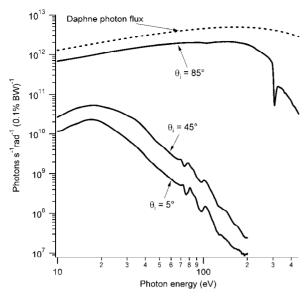
Figure 5: Number of reflected photons obtained by the reflectivity curves at incidence angle  $\theta_I = 85^{\circ}$ ,  $45^{\circ}$ ,  $5^{\circ}$ .
