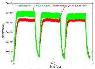
Figure 1: mean e-cloud linear density in the storage ring calculated for two different photoelectron yield values (0.2 and 0.1) with a reflectivity of 50%.
