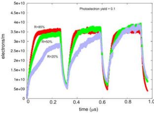
Figure 2: mean e-cloud linear density plotted changing the value of the reflectivity (85%, 50%, and 20%) with a photoelectron yield of 0.1.
