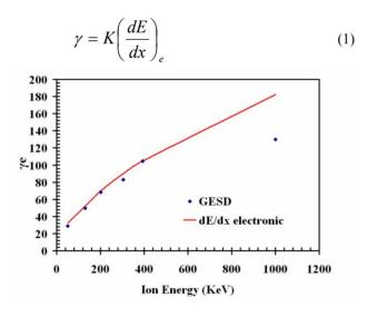
Figure 3: Electron Yield obtained with Gas-Electron Source Diagnostic at 88 degrees compared with the electronic stopping power normalized to 392.8 KeV.
