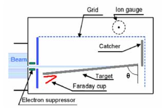
Figure 1: Gas-electron source diagnostic (GESD).
