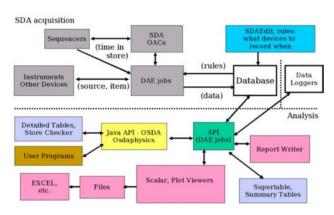
Figure 2: SDA data flow diagram.
