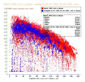
Figure 4: JAS Plot of Stacking Rate (A:STCKRT) vs. Stack size (A:IBEAM) in the Accumulator. The red points correspond to data collected during the entire month of March 2005. The blue points correspond to data collected during the first week of May 2005.
