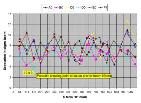
Figure 6: Proton antiproton separation from machine model (MAD).
