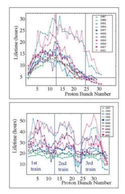
Figure 3: Proton lifetimes for 10 different stores. Top: central orbit. Bottom: before 1st cogging.
