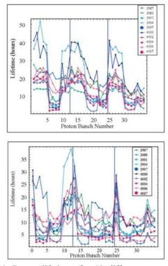
Figure 4: Proton lifetimes for 10 different stores. Top: Before the  $2^{nd}$  cogging. Bottom: before the ramp.
