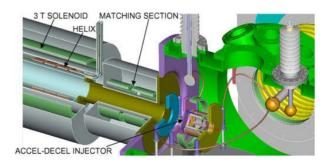
Figure 2: NDCX1c Experiment (cut-away view).
