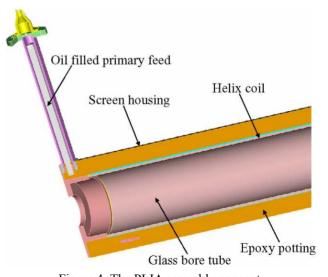
Figure 4: The PLIA assembly concept.
