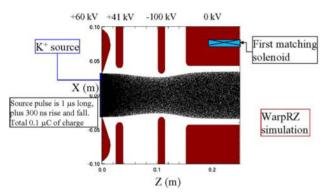
Figure 3: The Accel-Decel Injector.
