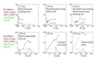
Figure 6: Snowplow mode with moderate compression.
