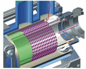
Figure 2: Termination resistor string for the oil dielectric helix.
