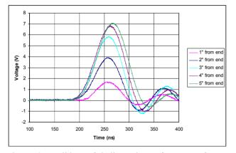
Figure 3: Buildup of helix voltage from transformer coupling with air dielectric.
