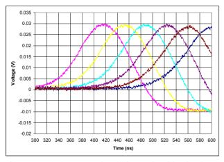
Figure 5:  $B_z(z,t)$  measured at 4" intervals with a hardware integrated B-dot loop with oil dielectric.
