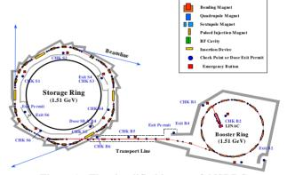
Figure 1: The simplified layout of NSRRC.
