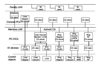
Figure 1: Schematic view of the SAGA-LS control system.
