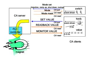
Figure 4: PV configuration of the magnet control system using ActiveX CA.
