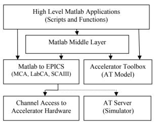
Figure 1: Software flow diagram.
