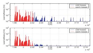
Figure 4: Example of protons losses in the LHC aperture along the IR7 region, for a vertical halo tracked at injection optics; Top: Only betatron cleaning (IR7) is considered; Bottom: The full LHC collimation system is considered.
