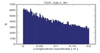
Figure 5: Longitudinal distribution of the horizontal halo protons absorbed at element TCLP.C6L7.B1, first horizontal primary collimator of LHC betatron cleaning insertion.
