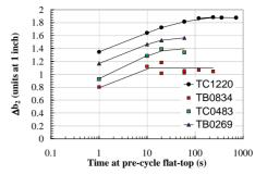
Figure 4:  $b_2$  drift amplitude after 30 min at injection for different pre-cycle flat-top durations (1 min back-porch) five Tevatron dipole magnets at 4.0 K.
