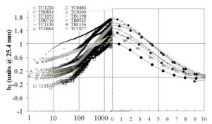
Figure 2: b<sub>2</sub> drift and snapback (vs time in sec) measured in 12 Tevatron dipoles after a standard pre-cycle at 4.0 K.
