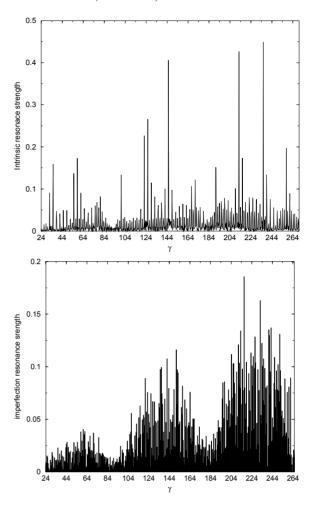
Figure 2: strength of intrinsic and imperfection spin resonance strength from injection energy to 250 GeV. They are the calculations of RHIC lattice without snakes and spin rotators. The intrinsic spin resonance strength is calculated with a single particle at an emittance of  $10\pi$  mm-mrad. The imperfection spin resonance strength is calculated with an rms vertical orbit distortion of 1mm.
