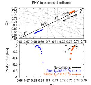
Figure 3: RHIC tune scans in the presence of four collisions. The top plot shows the working points with the location of the orbital resonance marked. The bottom plot shows the measured lifetime as a function of the working point.
