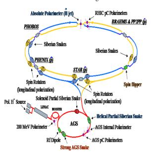
Figure 1: Polarized proton acceleration complex at Brookhaven National Laboratory
