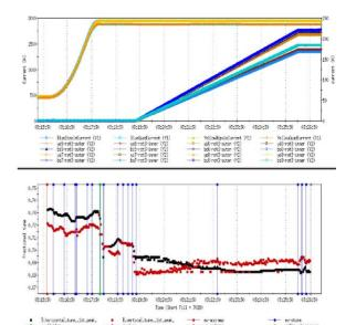
Figure 5: The top plot shows the RHIC main dipole and quadrupole current as well as the rotator current during the ramp. The lower plot shows the horizontal and vertical betatron tune during the ramp.
