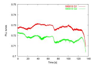
Figure 2: The tunes after the coupling corrections.
