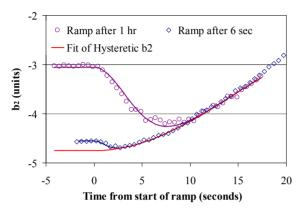
Figure 2. Plot of the measured  $b_2$  as a function of time on the energy ramp for two different length front porches.
