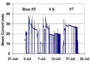
Figure 2: Average pulse current records for three experimental runs showing the best performance achieved using the original conditioning procedure.
