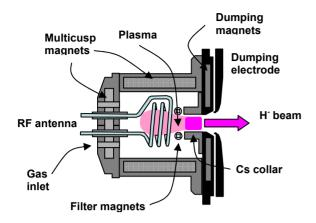
Figure 1: Schematic diagram of the SNS ion source.
