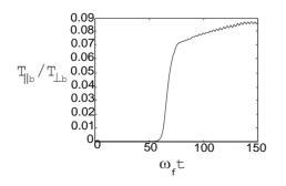
Figure 6: Plot of effective longitudinal temperature  $T_{||b} \equiv m_b < v_{||}^2 >$  as a function of time.
