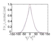
Figure 8: Plots of z-averaged longitudinal velocity distribution at times  $\omega_f t = 75$  (red dashed line),  $\omega_f t = 100$  (red dotted line) and  $\omega_f t = 150$  (solid blue line).
