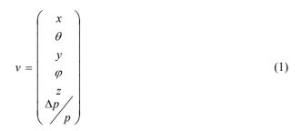
where x and y are the relative position to the center trajectory in horizontal and vertical directions respectively,  $\theta$  and  $\varphi$  are their derivative with respect to the trajectory position, z is the relative position to the synchronous particle and  $\Delta p/p$  is the momentum spread.
