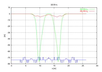
Figure 1: Second Order Chromaticity:  $\eta_x \partial \beta_{xy} / \partial \delta$ .
