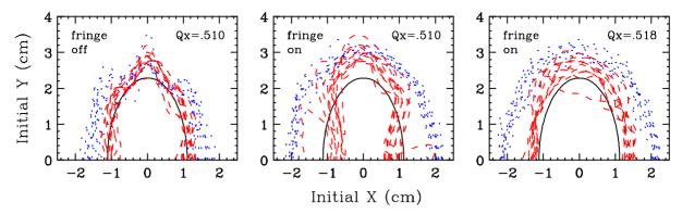
Figure 2: Evolution of HER dynamic aperture with quadrupole nonlinear fringe off and on at  $\nu_x = .510$  and .518.
