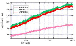
Figure 4: Example of matched readings for a pair of BPMs in the same shielding box (AMP11A and AMP11B).
