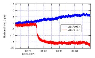
Figure 3: Smooth step change in the horizontal orbit at BPM AMP11B. Beam with no orbit correction.
