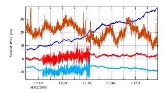
Figure 2: Examples of altered noise level affecting individual and group of monitors. Beam with no orbit correction.
