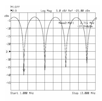
Figure 3: Frequency transfer function of the notch filter. Revolution frequency (2.72 MHz) and three harmonics of the filter are shown.
