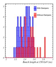
Figure 6: Bunch length at 150 GeV after coalescing for antiprotons, before and after the introduction of longitudinal damping.
