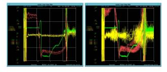
Figure 2: Longitudinal dampers on (left) and off (right) on a proton coalescing cycle. The yellow trace shows the longitudinal phase error of the central bunch.
