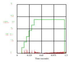
Figure 4: Transverse dampers allow long 8 GeV lifetime, essential for multibatch injection on NuMI cycle. The green traces show the beam current.
