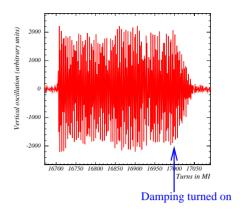
Figure 3: Damping of vertical injection oscillations. The initial oscillation amplitude is about 1mm.
