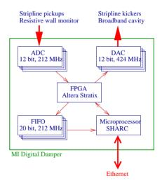
Figure 1: Schematic diagram of the main injector digital damper system.
