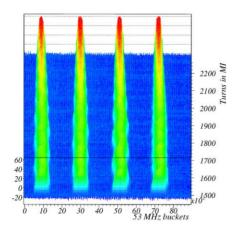
Figure 5: Longitudinal distribution of antiprotons bunched in 4 2.5 MHz bunches. The fourth bunch is damped.
