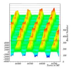
Figure 7: A coherent mode 1 instability on a NuMI study cycle. Plotted is the longitudinal phase error of each bunch, in arbitrary units, against turn and bunch number.
