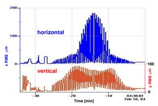
Figure 2: Horizontal and vertical RMS orbit response of all DPMs during IDFF recording for one of two electromagnetic undulator **UE212** at the surface/interface spectroscopy (SIS) beamline. Applying the estimated correction after each IDFF step restores the original RMS values within a few  $\mu$ m (see comb like shape). This IDFF table generation for one ID parameter takes  $\approx 20$  min. The FOFB is switched off during the entire measurement.
