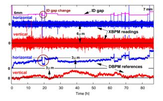
Figure 4: Slow XBPM feedbacks provide sub- $\mu$ m RMS photon beam stability ( $\sigma_x = 0.37 \ \mu$ m,  $\sigma_y = 0.5 \ \mu$ m) at the first optical elements of presently three beamlines (exemplified by the data taken at a PX beamline over 85 h of FOFB and "top-up" operation) [1]. For changing gaps <8.5 mm (top magenta line) the XBPM feedback corrects (see circles) for the residual distortions induced by the ID **U19** in the presence of IDFF tables as shown in Fig. 3.
