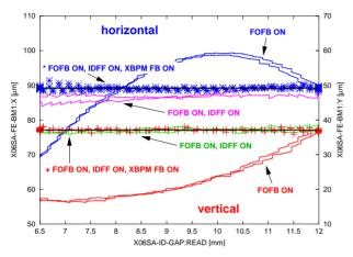
Figure 3: Stabilization of the horizontal and vertical photon beam position at the XBPM of a protein crystallography (PX) beamline  $\approx$ 8.6 m away from the source point of the in-vacuum ID **U24** during gap variations at a speed of 0.1 mm/s by means of FOFB, FOFB + IDFF tables and FOFB + IDFF tables + XBPM feedback.
