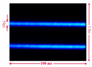
Figure 3: The longitudinal bunch motion measured by a streak camera. The total beam current is 200 mA and the fill pattern is uniform. The measured rms bunch length is 22 ps. The revolution period of TLS storage ring is 400 ns.
