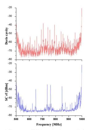
Figure 1: The spectra of BPM sum signal measured before and after the installation of SC rf cavity. The red line depicts the longitudinal beam spectrum measured when Doris cavities were used for particle acceleration. The blue line depicts the spectrum after the SC rf cavity was installed to replace the Doris cavities. The storage ring was uniformly filled and the total beam current was 200 mA.
