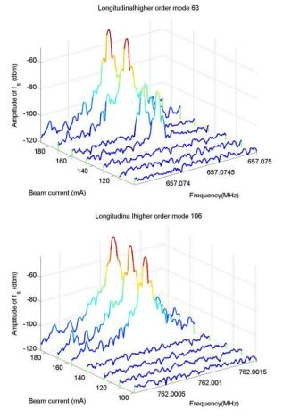
Figure 2: The dependence of the amplitude of synchrotron sideband on the total beam current. The top graph is the measurement for the longitudinal mode at 657 MHz, and the bottom is for the mode at 762 MHz. The threshold current is 130 mA for the longitudinal mode at 657 MHz and 140 mA for the mode at 762 MHz respectively.
