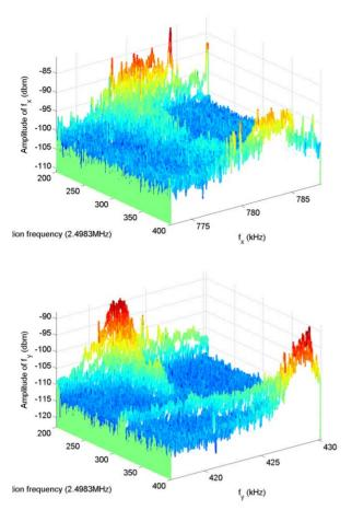
Figure 4: The spectrum of transverse BPM signal measured in user operation. The beam current was 180 mA and the transverse feedback was turned on. The top graph is the spectrum of horizontal BPM and the bottom is the one of vertical BPM.
