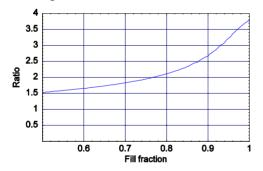
Figure 2: Touschek lifetime gain with respect to an unstretched bunch. The total current is held constant.
