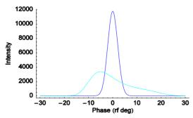
Figure 3: Line densities of unstretched (blue) and stretched (aqua) bunches in a uniform fill.
