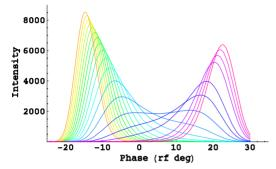
Figure 1: Line densities of bunches uniformly sampled along the length of an 80%-fill bunch train. The leading edge of each bunch is on the right and the progression of leading bunches to trailing bunches is from left to right. Each bunch is normalized to unity with respect to ring azimuthal angle.
