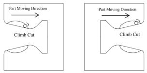
Figure 7: Start Chamfering at Different Pole End
