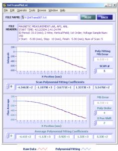
Figure 3: Field integral translation measurements.
