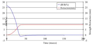
Figure 9: Eddy Current analysis of peak field change vs. time (dB/B) for a rapid field adjustment.
