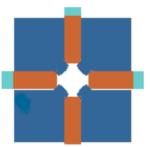
Figure 3: Method of correcting for temperature dependent vertical centerline shifts by using asymmetric vertical magnet temperature compensating steel
