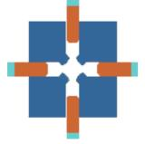
Figure 1: Method of achieving strength adjustment by uniformly retracting all four magnets in a PM Quad.
