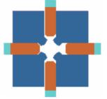
Figure 2: Method of shifting the horizontal magnetic centerline to the right by shifting a pair of magnets. (Highly exaggerated for illustration purposes.)
