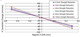
Figure 6: Magnetic centerline tuning curves for different strength retractions (0-10mm).
