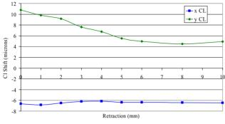
Figure 8: Magnet angle sensitivity. Angle of one magnet was changed by 5 degrees. Sensitivity is approximately 1 micron/degree.
