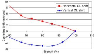
Figure 7: Pole positioning sensitivity. One pole was displaced 200 microns horizontally.
