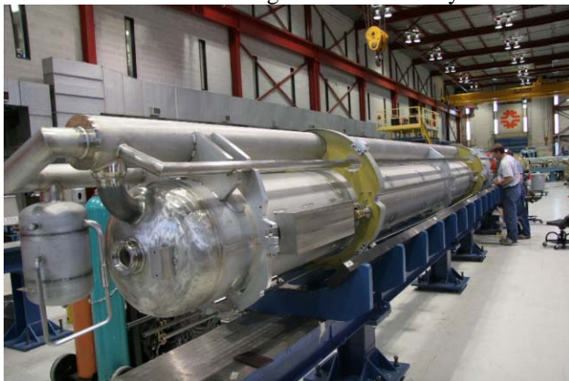
Figure 5. MQXA (KEK) quadrupole magnet completed as a Q1 cryo-magnet at Fermilab.
