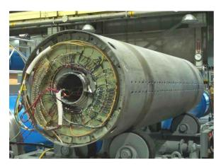
**Figure 2** The nearly completed cold mass before closure of the helium containment shell in the ends. The small holes along the length are for helium circulation.
