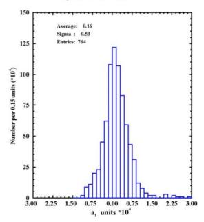
Figure 3 Final distribution of skew quadrupole in Tevatron dipoles after production shimming
