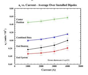
Figure 4 Current dependence of the average skew quadrupole for each third of the dipoles and the whole magnets ("combined")
