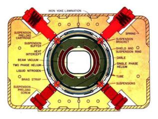
Figure 1 Tevatron dipole cross section
