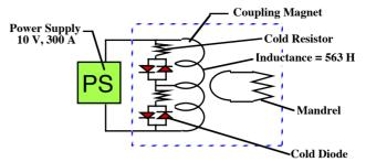
Figure 6. Circuit diagram for a single coupling magnet
