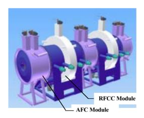
Figure 1. The MICE cooling channel.
