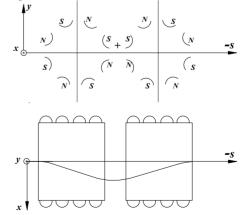
Figure 2: Octupoles installed rectangular to the beam trajectory. Trajectory is shown also. It runs ~in central part of each octupole ~along axis -s. For these purposes the yoke must have side openings there.
