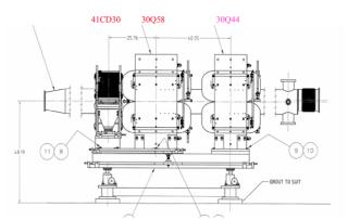
Figure 1: SNS ring doublet assembly [4].
