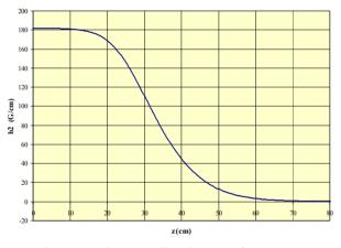
Figure 4: Linear gradient b2 vs. z for 30Q58.
