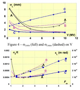
Figure 5 –  $\sigma_E/E$  (dashed) and  $\varepsilon_L$  (full) as functions of  $F_m$ .
