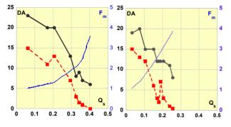
Figures 6-7 – Horizontal DA for structures A-B on energy (black dots) and at 6  $\sigma_E/E$  (red squares) as  $Q_s$  functions, and corresponding  $F_m$  (blue right scale).
