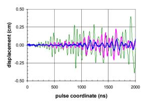
Figure 5: Horizontal beam displacement along the pulse when uniform radii of 0.445, 0.668, and 0.890 cm (green, red, and blue) are used over the transport channel.
