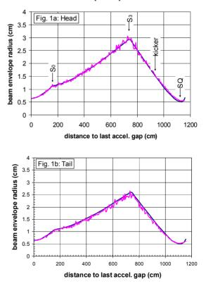
Figure 1: Comparison of beam envelopes calculated using LAMDA (blue) and LSP (red) at  $2x10^{-7}$  torr for the head (a) and the tail (b) of the pulse. Locations of the magnetic transport elements  $S_0$ ,  $S_3$ , kicker, and septum quad (SQ) are also marked in Fig. 1a.
