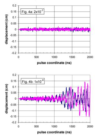
Figure 4: LSP results of horizontal (red) and vertical (blue) beam displacement, observed at the septum quad, due to ion-hose effect at pressure levels of (a)  $2x10^{-7}$  and (b)  $1x10^{-6}$  torr.
