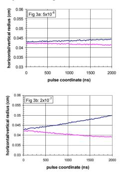
Figure 3: Horizontal (red) and vertical (blue) beam radii during the beam pulse at the final focus for pressure levels (a)  $5x10^{-8}$  and (b)  $2x10^{-7}$  torr.
