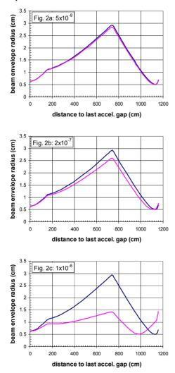
Figure 2: Beam envelopes for the head (blue) and for the tail (red) between the last accelerator gap and the septum quad at different pressure.
