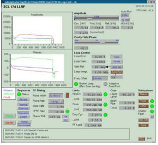
Figure 2: Low Level RF screen showing the RF amplitudes (Forward blue, transmitted red, reflected green) during a quench event for an SNS superconducting cavity. During the quench the loaded Q drops to about  $3x10^5$  and the unloaded  $Q_o$  to  $4x10^5$ .
