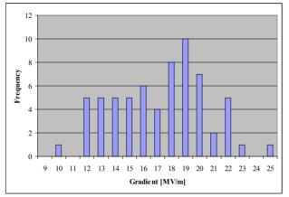
Figure 4: Distribution of maximum gradients achieved in the SNS superconducting cavities so far (65 out of 81) at 4.2 K in open loop at 1.3 msec pulse length at 10 pps. The overall average value is 17.8 MV/m.
