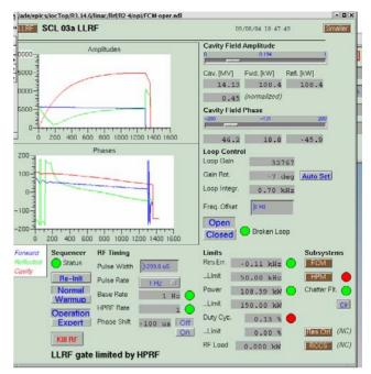
Figure 1: Low Level RF traces of forward (blue), reflected (green) and transmitted (red) amplitude (above) and phase (below) for a SNS superconducting cavity.
