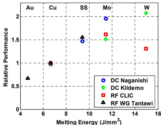
Figure 5: Material dependence of the maximum achievable surface field [7, 8, 9, 10].
