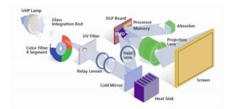
Figure 8: Display Wall projection engine.
