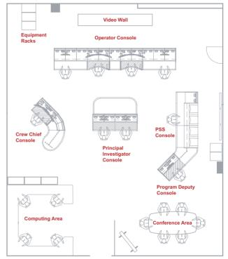
Figure 7: New control room layout.
