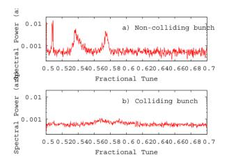
Figure 1: Bunch spectra for a) non-colliding, and b) colliding LER bunches with a 2-bucket (4 ns) separation from the preceeding bunch
