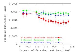
Figure 8: Specific luminosity of 2-bucket colliding observer bunch, and those of 3- and 4-bucket bunches, for different currents of the test bunch preceeding the 2-bucket observer bunch
