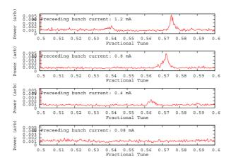
Figure 5: Bunch spectra of the non-colliding observer bunch. Figures a-d show the spectrum for the observer bunch at different bunch currents for the preceeding bunch (the test bunch).
