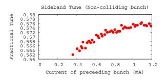
Figure 7: Sideband tune of non-colliding observer bunch for different currents of preceeding bunch
