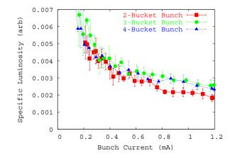
Figure 4: Specific luminosity as a function of bunch current for the 2-bucket colliding test bunch, as well as that for nearby 3-bucket and 4-bucket bunches. Each point is the average of 4 consecutive measurements; error bars are  $1-\sigma$ statistical error bars.
