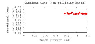
Figure 3: Sideband tune of non-colliding test bunch as a function of test bunch current
