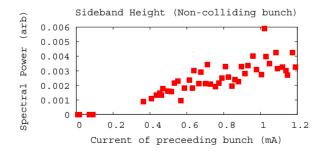
Figure 6: Sideband peak height of non-colliding observer bunch for different currents of preceeding bunch
