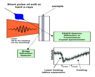
Fig. 1. Schematic of laser-x-ray pump probe
