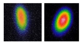
Fig. 3a.: X-rays generated from the velocity compressed, 300fs, electron beam vs. (b) uncompressed 5 ps beam.
