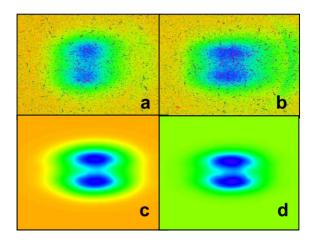
Fig. 4: K-edge radiography through U. 4a. PLEIADES tuned to 115 keV k-edge, for on axis x-rays, which are abosorbed by k-edge. 4b. PLEIADES tuned away from k-edge, on axis x-rays begin being transmitted through foil. 4 c and d are BLOWER simulations.
