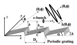
Figure 1: The SPR scheme. An electron bunch is traveling at an axial velocity  $v_x$  above an echelle grating of period  $D_g$ .
