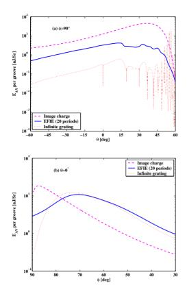
Figure 2: Comparison of average first-order radiated energy per groove by the 20-period grating (solid line) with the energy per groove by the image-charge model (dashed line) and by the infinitely long grating assumption (dotted line). The energies are plotted versus  $\theta$  when  $\phi = 90^{\circ}$  (a) and versus  $\phi$  when  $\theta = 0^{\circ}$  (b)
