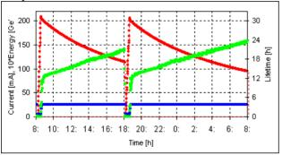
Figure 3: Typical current and lifetime at ANKA.
