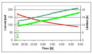
Figure 9: Current and lifetime with phase modulation on (upper dark green and red curve) and lifetime with phase modulation off (soft green).
