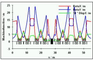
Figure 10: Beta Function for the planned low beta optics.
