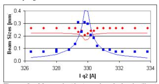
Figure 8: Measured (dots) and calculated (lines) horizontal (red) und vertical (blue) beam sizes.
