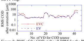
Figure 8: RMS of the COD at the all BPM for the PF ring.
