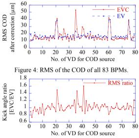
Figure 5: RMS ratio of the kick angles of the steering magnets.
