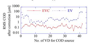
Figure 7: RMS of the COD at the constraint point for the PF ring.
