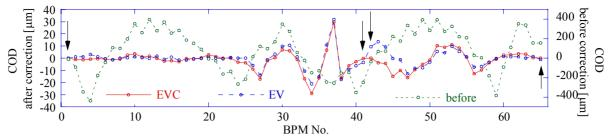
Figure 6: The typical vertical CODs before and after correction by the EVC and EV.
