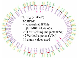
Figure 2: Configuration of the BPM and vertical orbit correction system at the PF ring.
